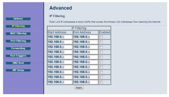
Figure 17. Example of IP Filtering Page
