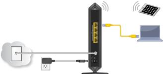
For a wired connection, use an Ethernet cable to connect a computer to an Ethernet port on the modem router.
