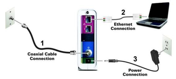
Figure 4: SB8200 Connection Diagram
