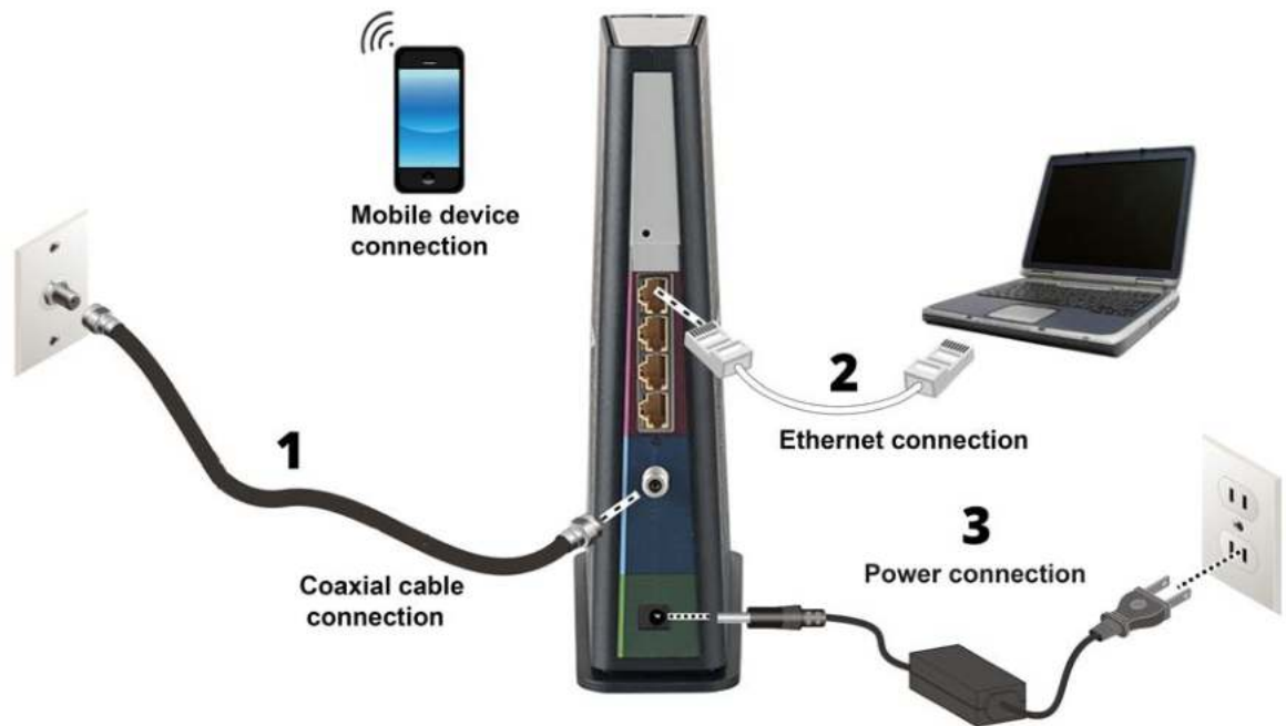
Figure 4: SBG8300 connection diagram
