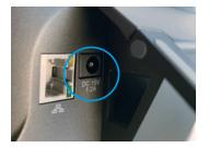
A Remove the existing power cord from the back of the touchscreen by unplugging it and routing it through the stand.
