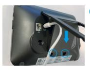
Replace the stand on the back of your touchscreen, slide it down, and screw the two small Philips screws back on the bottom of the touchscreen under the stand.
