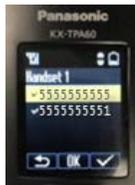
7. Place a check mark next to the name of each Handset that will be allowed to receive calls for the number. In this example, Handset 1 and Handset 2 will receive calls for TN 555-555-5555.
