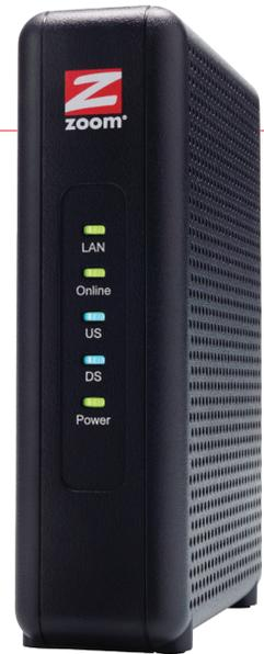
The Zoom Model 5345 cable modem meets the cable industry's DOCSIS 3.0 standard for speeds up to 343 Mbps, and also works with lower-speed DOCSIS 2.0 and 1.1 services. Full-Band Capture Digital Tuning allows service providers to offer more channels and accelerate downloads. The Model 5345 has been tested and certified by CableLabs® to work with nearly all U.S. cable services.
